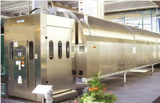
The next big step forward came with the design of the continuous batch washer. This consisted of a tube some 1.5 metres in diameter divided into compartments by a helical scroll rather like an Archimedean screw. Instead of rotating completely like a washer extractor the CBW rocked through an arc to create the necessary mechanical action.
